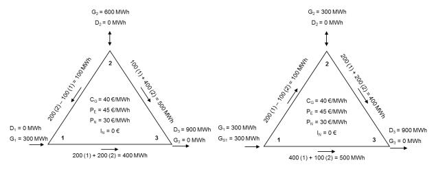
Figure 5 Alternative 2a: Second period – storage feeding back to the grid.
